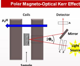
The sample is magnetized in a magnetic field created by an electromagnet. Generalized ellipsometry in the polar configuration (incident light parallel to the magnetic field) can be performed by shining light through a hole in the magnetic pole piece.
