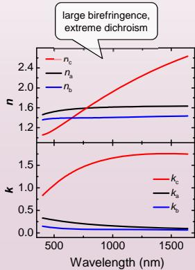
Principal refractive index  $n_i$  and extinction coefficient  $k_i$  along axes  $i = a, b, c$  of cobalt slanted columnar thin film depicted in the SEM.
