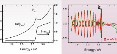
A significant difference between the parallel and perpendicular dielectric function was found for ZnMnSe.
