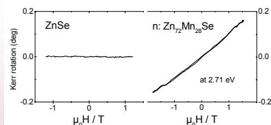
MOGE measurements in quasi-Kerr configuration for ZnSe, and Zn<sub>72</sub>Mn<sub>28</sub>Se. The Zn<sub>72</sub>Mn<sub>28</sub>Se sample shows a paramagnetic response for a photon energy corresponding to the band-to-band transition, while in ZnSe no Kerr rotation is detected.
