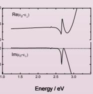
12 meV conduction band splitting energy detected in  $\varepsilon_{\parallel}$  and  $\varepsilon_{\perp}$  at  $\mu_0 H = 1.8$  T.
