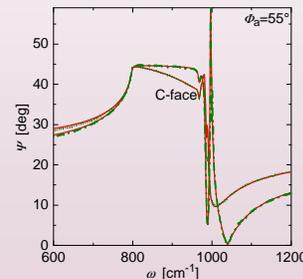
Fingerprint of graphene at the rest-stahlenband of SiC - more dominant for C-face grown graphene
