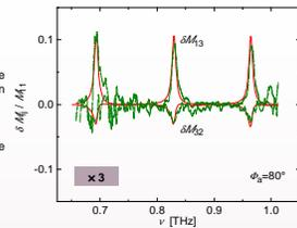
Non-zero Mueller matrix  $M_{2,22}$  difference spectra for  $\delta B \sim 3.4$  T in the THz region allow the determination of the graphene free-charge carrier effective mass
