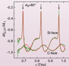
Fabry-Pérot interferences (arrows) originating from the SiC substrate are damped out for C-face grown graphene
