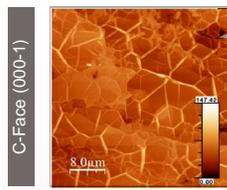
AFM topography of graphene on C-face, showing typical "giraffe pattern"
